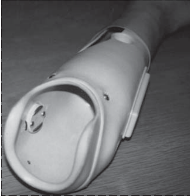
Fig. 3-52. Myoelectric electrodes embedded in a prosthetic socket.
